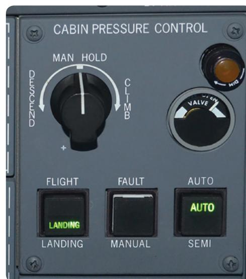
Figure 1.7 – Pressurization Panel was not reset back to auto.
